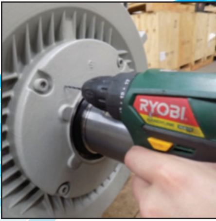
9) Drill hole with 2.5mm Steel drill bit.
