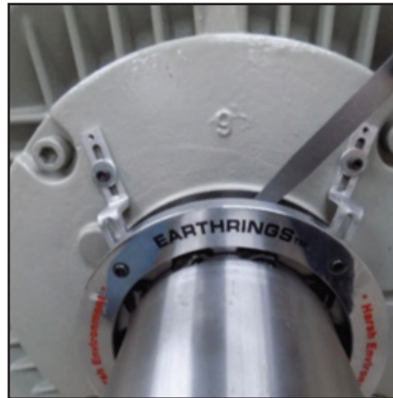
15) Use 1mm Feeler gauge to check Earthing has a minimum of 1mm gap from the shafts shoulder, plus also check that Earthing is vertically straight at 90 degree angle / parallel with the shaft and grease cover / endshield.
