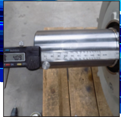
10) Check Depth of hole with Vernia and make sure you have not drilled completely through. (If you have remove endshield or grease cover, remove grease clean bearing and Grease cover with thinners, re-grease bearing and fit Grease cover back in place)
