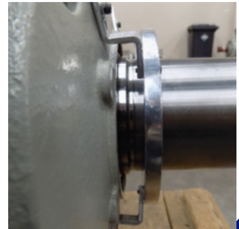
15) Use 1mm Feeler gauge to check Earthing has a minimum of 1mm gap from the shafts shoulder, plus also check that Earthing is vertically straight at 90 degree angle / parallel with the shaft and grease cover / endshield.
