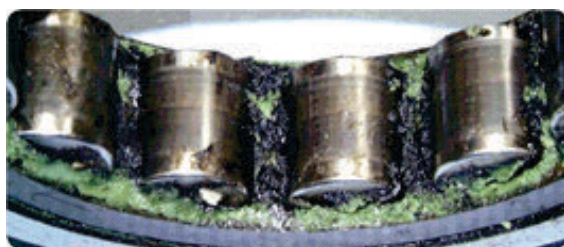
Hardening of Grease , stops Relubrication.
