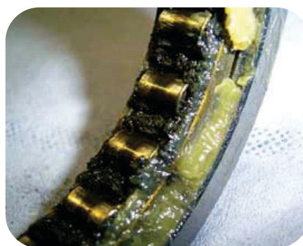
Hardened oxidation of Grease stops new Grease entering Rollers
