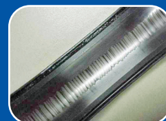
The “Picket Fence” pattern is due to shaft voltages.
