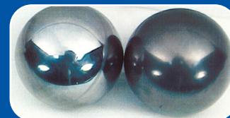
The darkened finish was caused by electric currents.
