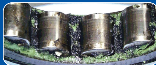
Eddy Currents Damaging Bearing Grease - Increasing Service Intervals.
