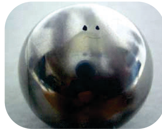
Light Brown marks and Pitting
