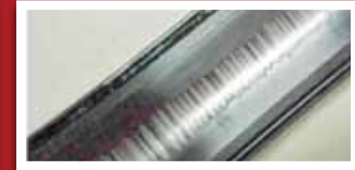
Damaged grease & Bearing fluting, "washboard" pattern on bearing race
